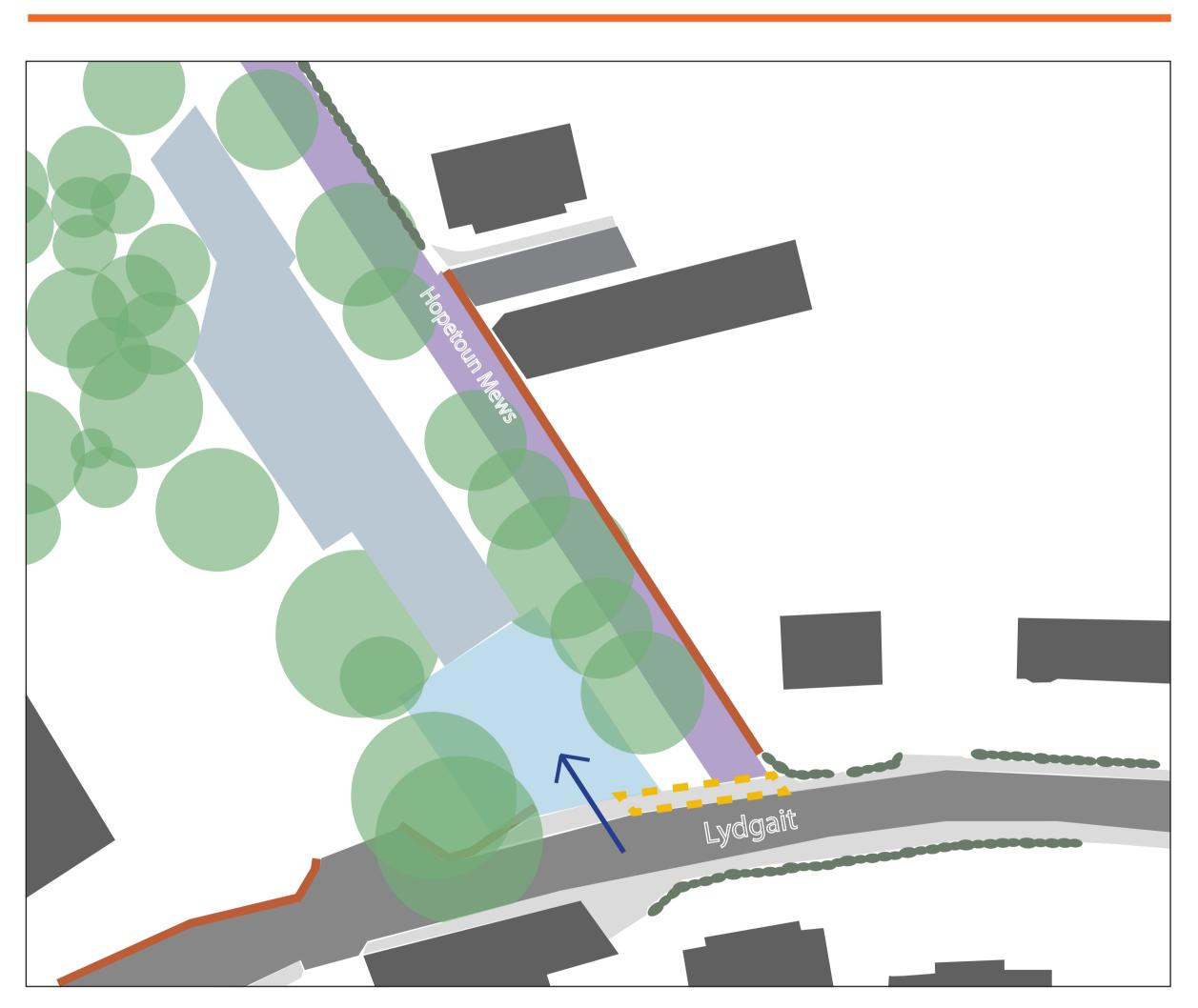
The existing vehicular junction between Lydgait and Hopetoun Mews could be narrowed and a new section of footpath proposed across the junction. This could help provide a safe and unobstructed entrance for padestrians and cyclists.
