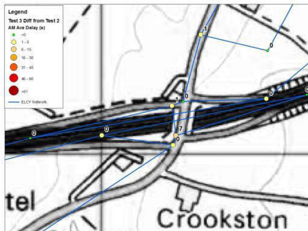
Figure 70. Test 3 vs Test 2 junction delay – Salters Road
